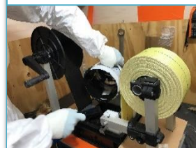
Fig. 6: BOBIPREG - 3X specific machine for Kevlar® tape impregnation
