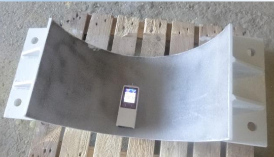
Figure 1: Roughness measurement on support sandblasted
