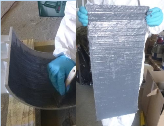
Figure 2: Filler application on support Figure 3: Filler application on ROLLERKIT®
