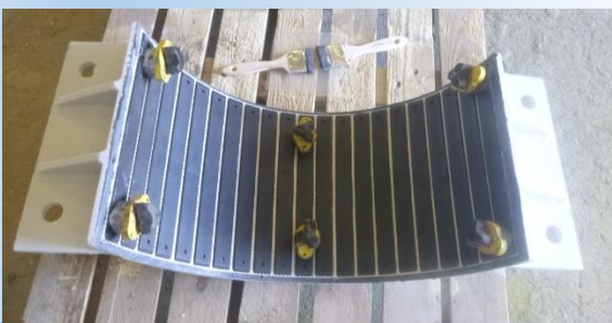
Figure 4: ROLLERKIT® fixing on support using magnets
