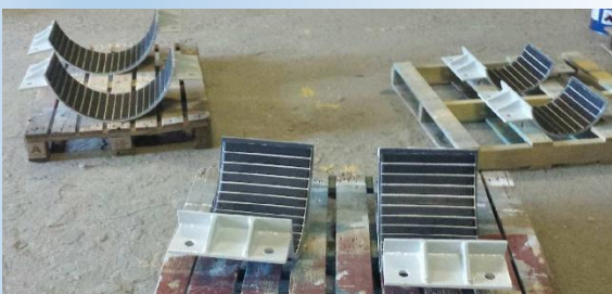
Figure 5: General view of the 6 supports protected with ROLLERKIT®
