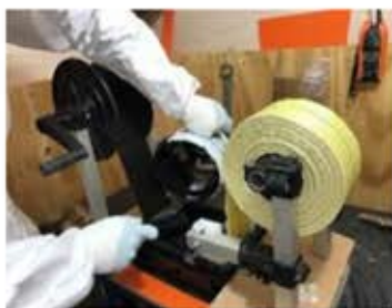
BOBIPREG - 3X specific machine for Kevlar® tape impregnation ●
